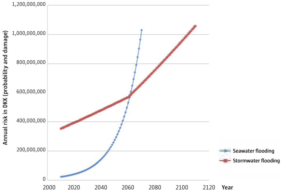
Figure 3: A risk area has been calculated for flooding from the sea. The index is calculated as the probability of an event times damage caused in the event. Table 3 shows the risk area as the number of million Danish kroner of damage that will occur in 10-year intervals.
