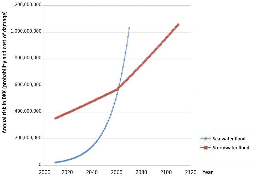
Figure 6. Risk of flooding from rain and seawater
