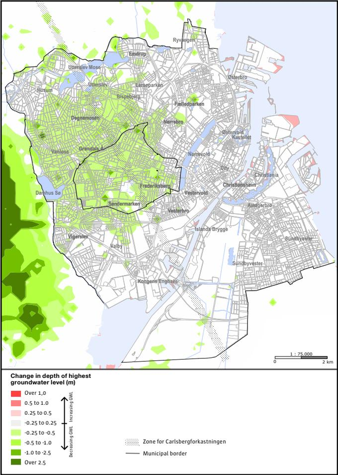
Figure 1: Change in depth of highest groundwater level—2060
